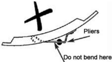
Remove the lid and gasket to ensure that the spring is protruding from the edge of the flange by 1 mm. (Fig. 5.).
