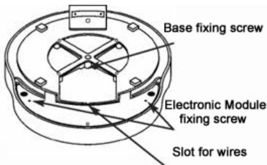
Disconnect the push on terminals from the wiring of the base and the heater element.
