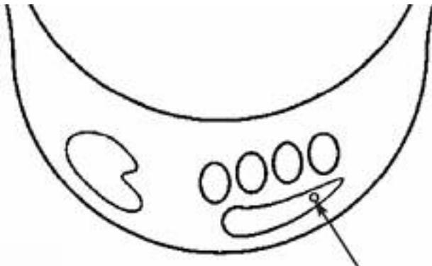
Fill to water level with **de-ionised/distilled** water (0.75L). Put on the test lid with pressure gauge and digital thermometer connected. Then open the vent valve.
