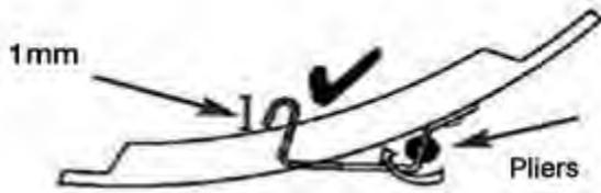
Ensure the lid is flat and stable and apply the pliers vertically. Locate the pliers onto the back edge of the spring and twist inwards carefully. Do not buckle the spring. Check visually and measure the distance again.
