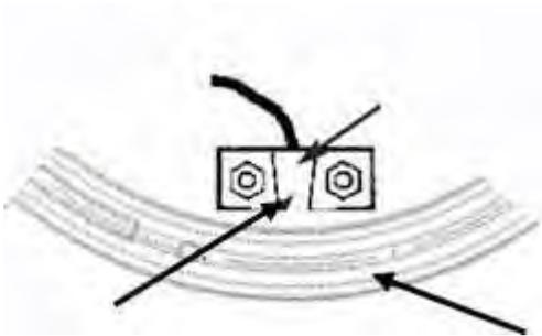
Position Thermistor pocket to create gap - min 0.5 mm; max 1 mm - between pocket & element
