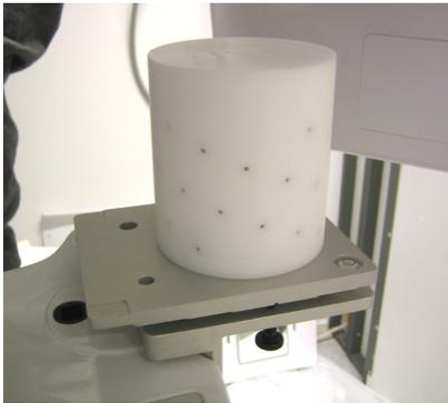
4. Install the 3D calibration phantom.
