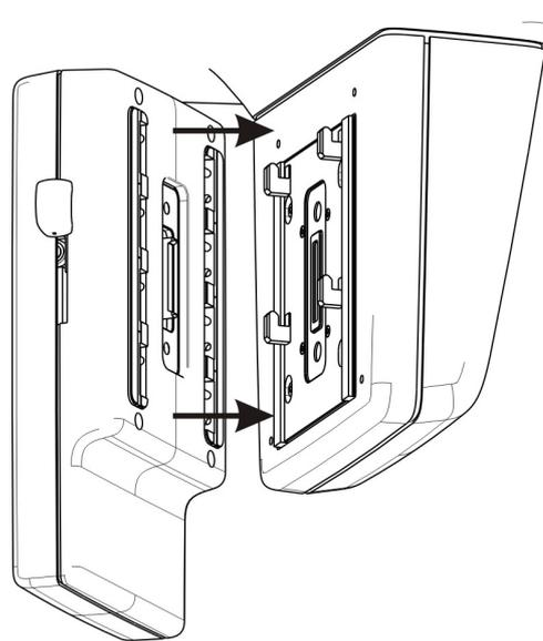
2. Pull the sensor downwards firmly until it stops and then slide the locking knob down on the side of the sensor to lock the sensor in position.
