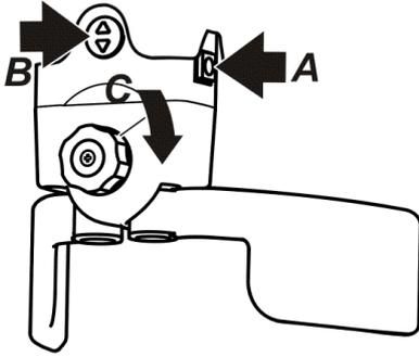
7. With the patient's head already at the correct tilt, bring the head support unit toward the patient by depressing the A buttons on either side, and up and down by depressing the B button. Releasing the buttons locks the assembly. Next, turn the C knob to close the temple supports.
