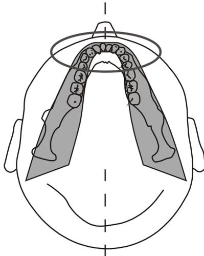
Image Layer corresponds to the thickness of the x-ray capture area (focal trough) in relation to the position of the teeth. Typically, this trough completely encompasses the anterior teeth. However, in the case of a retruded bite, the teeth may be behind the trough. Conversely, with the protruded bite, the teeth may extend in front of the trough. The result of either is a non-optimal image.
