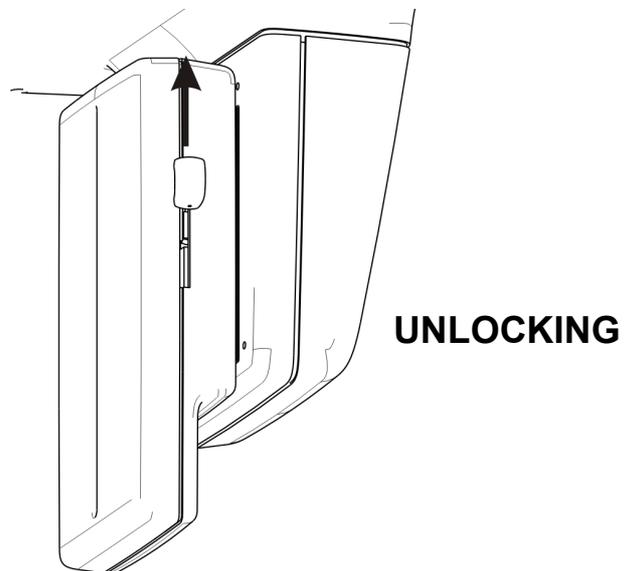
2. Slide the sensor up and remove it.
