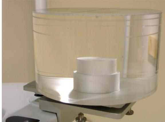
2. Ensure that QC phantom is aligned with the spirit level on the phantom base. If it's not, level it using the screws on the bottom of the phantom base.
