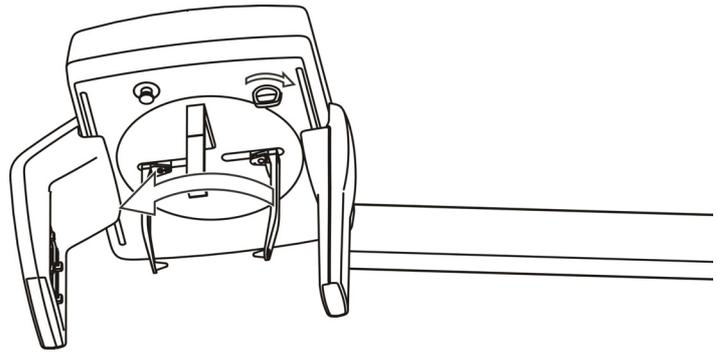
*Figure 1.2* Locking lever (1), ear holder brake (2)
