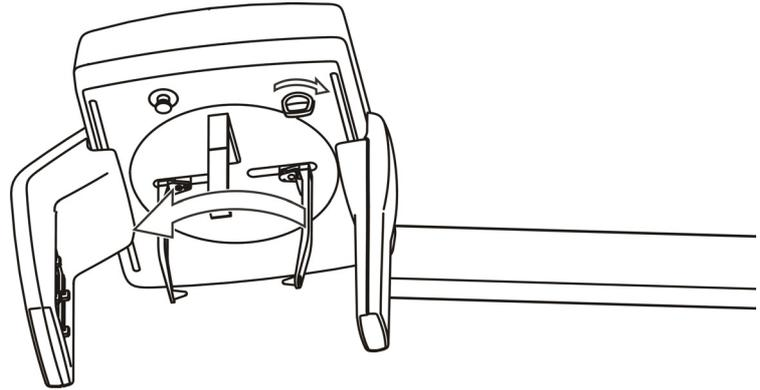
Figure 1.3 Locking lever (1), ear holder brake (2)
