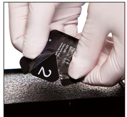
Figure 9. Ejecting a Plate into the Plate Transfer Box
