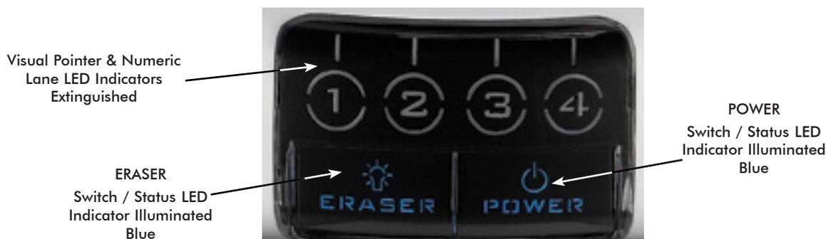
Figure 4. READY Mode Front Panel Indicators
