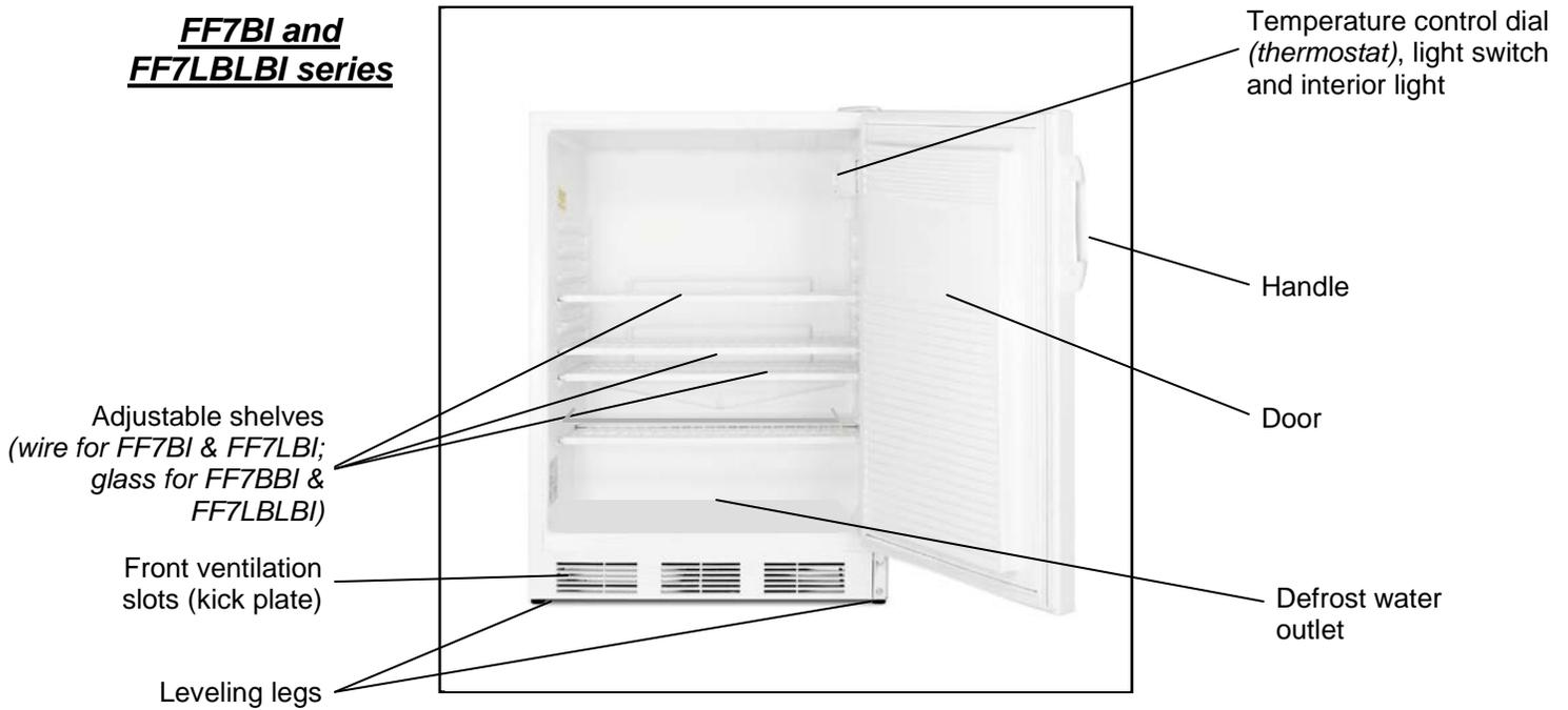
*NOTE: Lock on models FF7LBI and FF7LBLBI is located on the front of the door, near the top center.*
